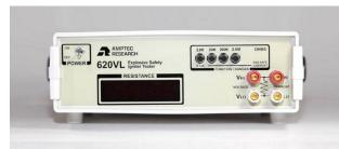
The Amptec 620VL Failsafe Ohmmeter is used for testing squibs, explosive bridge wire, flares, and similar components. This product was specifically designed in the event the meter should fall or break, it remains "inert" or safe for ultra-safe testing. The 620VL comes standard with an RS232C interface and runs on 4 rechargeable NICAD batteries.
